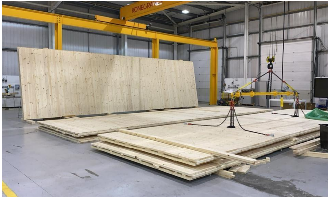
12m x 3m x 100mm CLT Wall Panels
